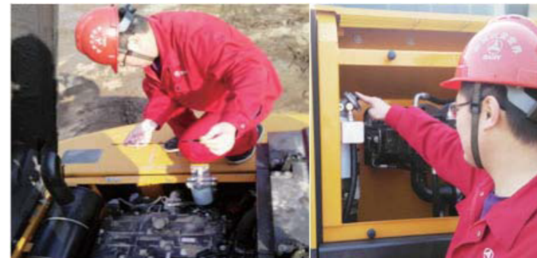
Inspect the situation of engine oil
