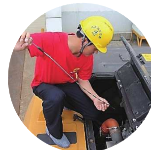
Inspect the situation of engine oil
